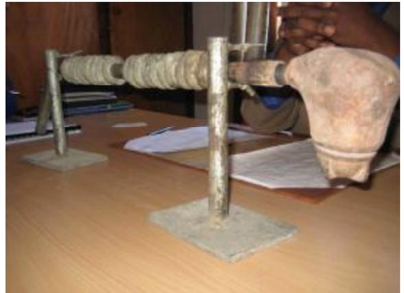
Fig 10 and Fig 11. Locally made metal retorts that owned by artisanal and small scale miners
