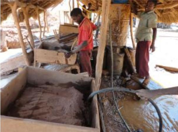
Fig 2. Gold ore sluicing by using constant flow employing the siphon method at Katente mining center, Shinyanga Region
